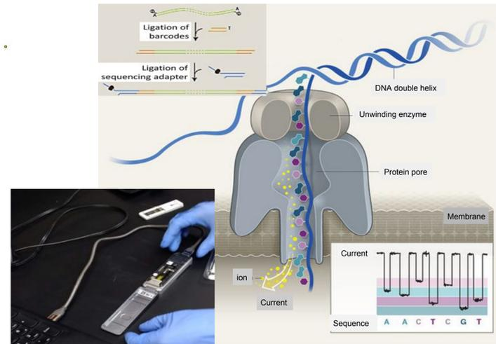
**Figure 3.** The ONT minION flow cell and illustration of how the minION flow cell operates. *Nature* 2017, GTEx Consortium.
