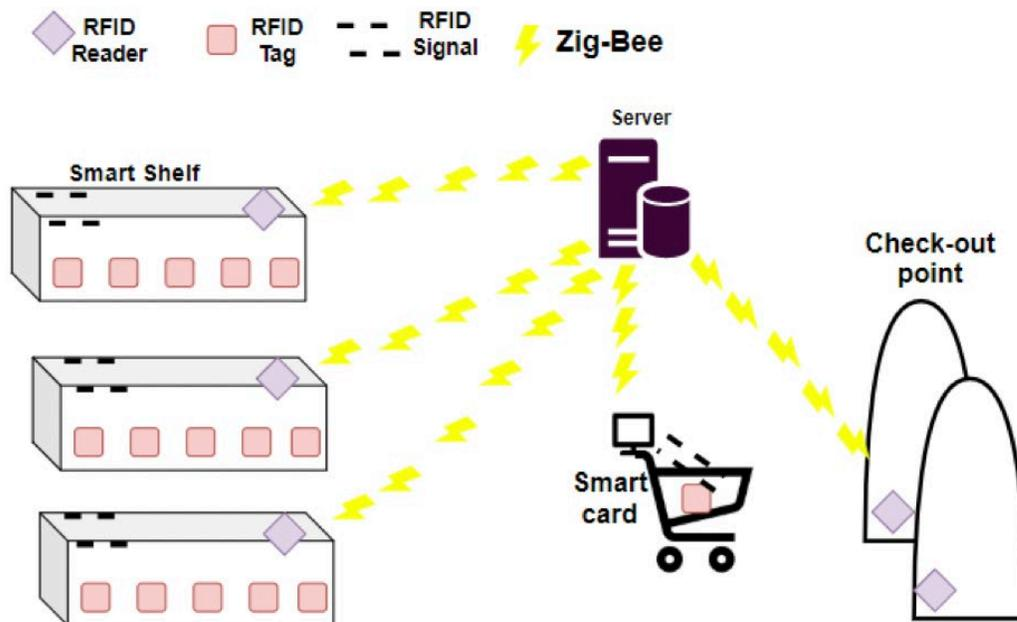
**Figure 4: Design of the smart card with the supermarket**
